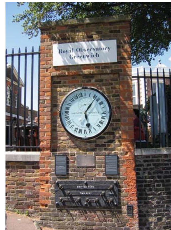
Shepherd Clock: 12 noon points to the bottom. The minutes are inscribed on a different scale. The time is 6 minutes after 11:00 am local.
